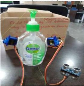
The HC-SR04 ultrasonic sensor with the help of servo motors can he handled as automatic sanitizer dispenser. The hands should be waved near the ultrasonic sensor and the sanitizer instantly will get ejected into the hands.
