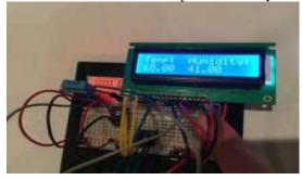
The temperature sensor is used to measure the temperature of the body which is connected to the Arduino. It is used to display the temperature on
